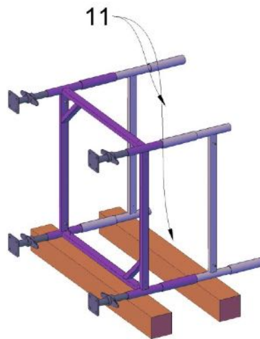
Fig. 11 – insertion of the base frame in the base jacks
